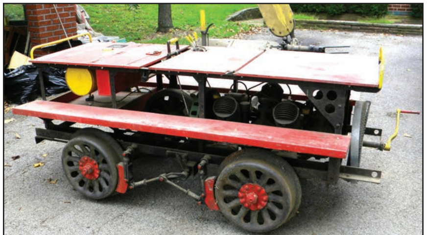
As-bought condition. Note the wheels are under the running boards on my narrow gauge #34.
