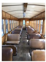
One coach car without trucks. Car was constructed from a D&RGW 6500 series flat car by the Cumbres and Toltec Scenic Railroad in the early 1980s. The frame is steel with a composite car body. The car has recently been removed from service and has the following:
