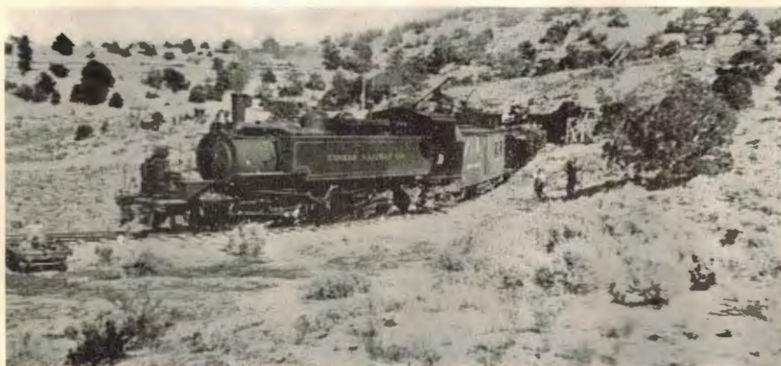
Pulling Out of Thimble Rock Mines, on a 7\frac{1}{2} Per Cent Grade and 66-Degree Curve
