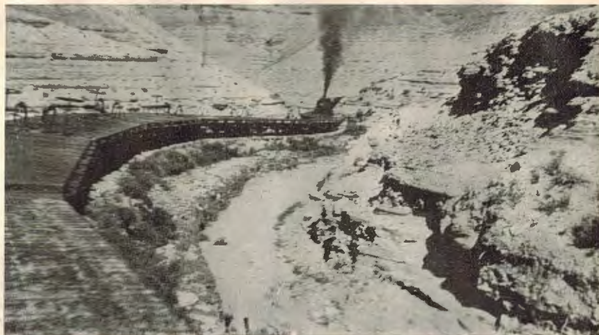
Pushing Empties for the Mines up the 5 Per Cent Grade Between Rainbow Junction and Rainbow
