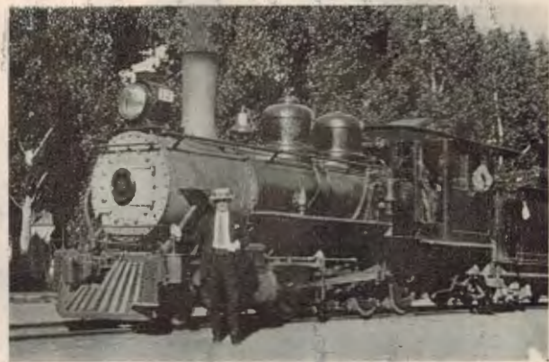
Consolidation Type Locomotive, Originally Built by The Baldwin Locomotive Works in 1896, and Purchased by the Uintah Railway in 1917
