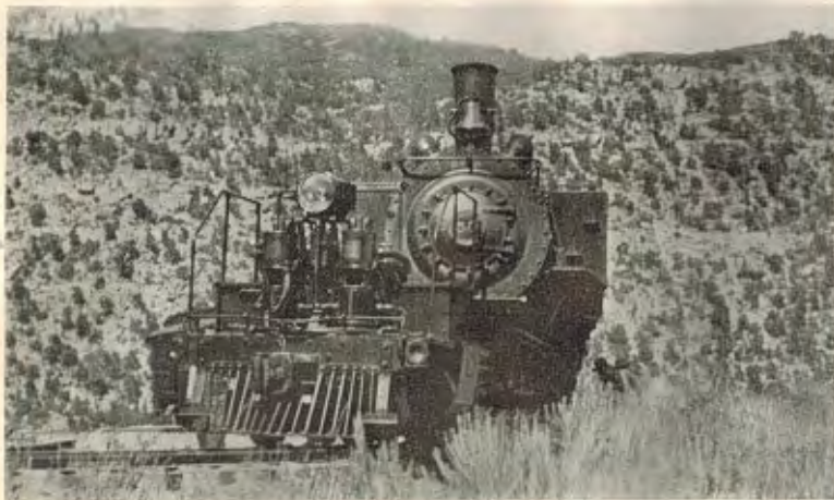
The New Articulated Locomotive on the 66-Degree Curve and 7\frac{1}{2} Per Cent Grade at Moro Castle
