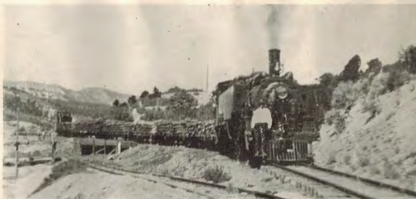
East Bound at McAndrews Station, Hauling 250 Tons on a Grade of 5 Per Cent
