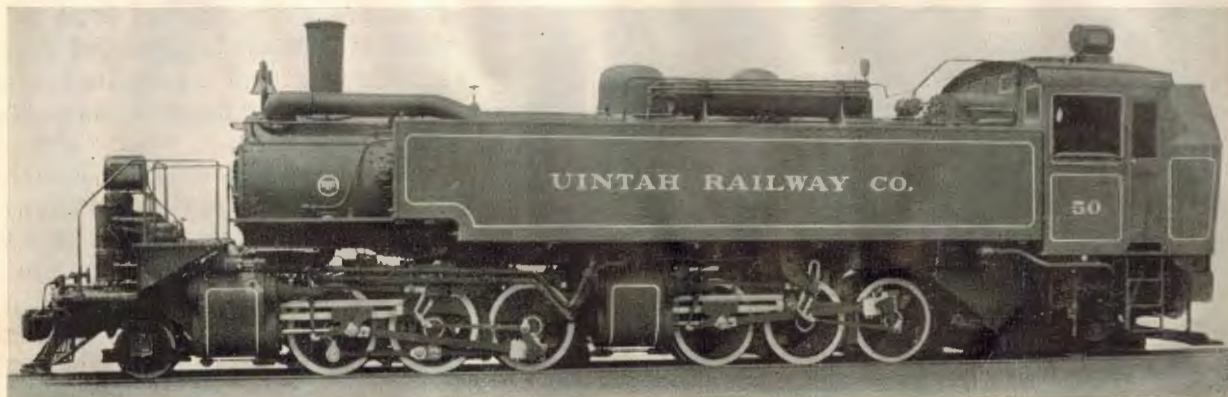
Right and Left Hand Views of the New Articulated Locomotive
